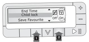
press the Ok button to enable this option. The corresponding icon changes your status from Off to On and the following message appears on the display: «Press And together for 5 seconds to unlock machine.».
