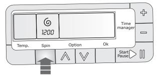
Press the **Spin** button repeatedly to change the spin speed, if you want your laundry to be spun at a speed different from the one proposed by the washing machine.
