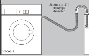
When discharging into a standpipe ensure that the top of the standpipe is no more than 90 cm (35.4'') and no less than 60 cm (23.6'') above floor level. The drain hose may be extended to a maximum of 4 metres.
