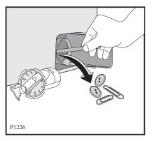
replace the filter into the pump paying attention to insert it properly. When done, screw it firmly
