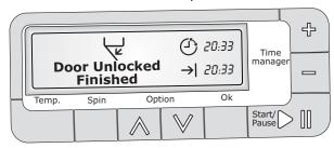
If your laundry is not removed during 10 minutes after the programme is finished, the backlight of the display switches off and the energy saving system will be enabled.
