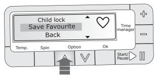
• press the **Ok** button to save the selected programme. On the display appears the message «Saved» in highlighted mode.
