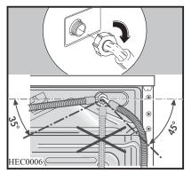
3. Set the hose correctly by loosening the ring nut. After positioning the inlet hose, be sure to tighten the ring nut again to prevent leaks. 4. Connect the hose to a tap with a 3/4" thread. Always use the hose supplied with the appliance. The inlet hose must not be lengthened. If it is too short and you do not wish to move the tap, you will have to purchase a new, longer hose specially designed for this type of use.
