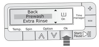
Once you have completed the selection of the options, press **Temp.** or **Spin** buttons or simply wait 10 seconds to return the display in the default status.
