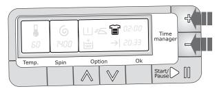
This function allows you to modify the washing time, automatically proposed by the washing machine. By pressing the «**Time manager** buttons «**+**/**-**» repeatedly, the duration of the washing cycle can be increased or decreased.
