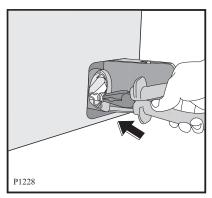
• replace the emergency emptying cap into the filter cover and fix it firmly
