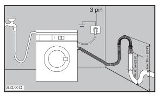
An additional drain hose and joining piece is available from your local Service Force Centre. The joining piece must have an internal diameter of 18 mm.
