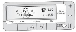
When the machine performs the washing phase the display shows also some animated bubbles that simulate the moving of the water.
