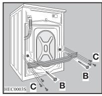
5. Remove the bracket **D** and refit the six smaller bolts **C** and slide out the relevant plastic spacer **E**.
