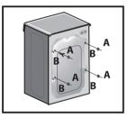
**Step 3**. Remove the 4 retaining screws at the rear of the machine, as indicated in the image on the left. Use the blanking plugs provided in the instruction booklet pack to cover the holes once the screws have been removed.
