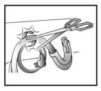
**Step 2**. Carefully cut through the hose-retaining clip at the rear of the machine, taking care not to cut the hose itself.
