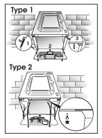
**Step 4**. Tilt the machine forward and apply the insulation base panel (corrugated plastic) to the base of the machine.
