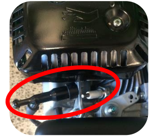
Disconnected spark plug
