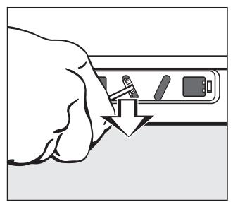
Insert a screwdriver into the notch of the left opening and pull downwards. The door will now open.
