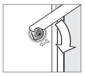
Turn the right shipping strut counterclockwise 90° with the enclosed combination wrench and.
