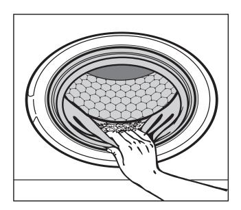
Check the folds of the door seal for any small articles which may have been trapped.
