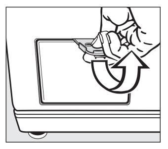
To clean the lint trap, remove the tool from behind the detergent dispenser drawer. If the main drain hose is clogged, water will be retained in the machine **(a maximum amount of 6.5 gal [25 I])**.
