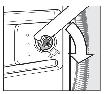
■ Turn the right shipping strut counterclockwise 90° with the enclosed combination wrench.
