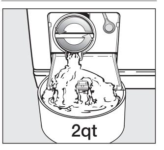
Turn the lint trap lid counterclockwise. Do **not** remove it. About 2 quarts of water will drain out of the hose.
