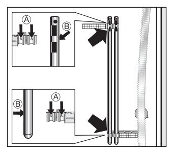
Fasten the shipping struts at the rear side of the washer. Take care to insert the drill holes (B) onto the spigot (A).
