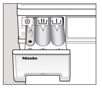
Place the recommended amount of detergent into the main wash compartment <u>U</u>. If "Heavy Soil" is selected, add 1/4 of the total amount of detergent to the <u>U</u> compartment. Place fabric softener or liquid starch in compartment <u>&</u>. 7. Select Delay Start (if needed)
