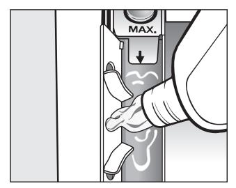
Add the fabric conditioner or liquid starch to compartment <sup>®</sup>. Do not exceed the maximum level mark.
