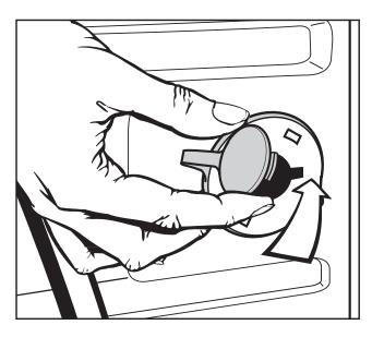
■ Fit the covers on to the two holes. Then plug the holes as shown with the caps.
