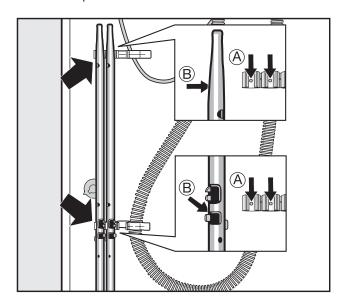
■ Secure the transit bars to the back of the washer-extractor. Make sure that holes **B** are fitted over retainers **A**.
