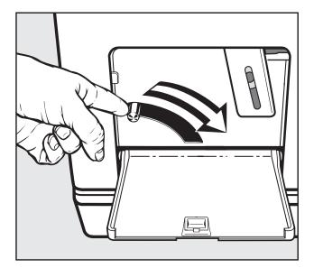
■ Push the emergency drain lever downwards (see illustration) and hold until no more water runs out.
