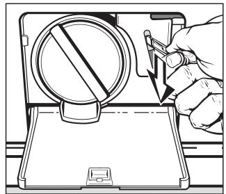
■ Use a spoon handle to pull the emergency release downwards (see arrow). The drum door will open.
