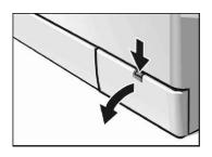
The water in the drum should be drained first before cleaning the drain pump. Have a suitable container ready.
