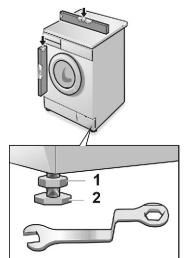
All four appliance feet must be firmly on the ground. The washing machine must not wobble
