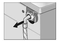
☐ Disconnect the hose from the back of the washer-dryer.
