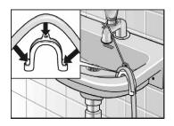
Drainage into a wash basin( The hose elbow is in the drum).
