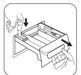
Remove the drawer by pressing the catch downwards and by pulling it out. Flush it out under a tap, to remove any traces of accumulated powder.
