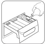
Pull out the dispenser drawer until it stops. Measure out the amount of detergent required, pour it into the main wash compartment (III) or in the appropriate compartment if the selected programme/option it requires (see more details in "Detergent dispenser drawer"). If required, pour fabric softener into the compartment marked (the amount used must not exceed the «MAX» mark in the drawer). Close the drawer gently.
