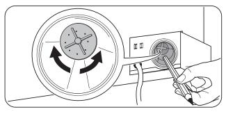
Check carefully whether the pump impeller rotates (it rotates jerkily). If it doesn't rotate, please contact your Service Centre.
