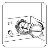
Replace the filter into the pump by inserting it correctly into the special guides. Screw the pump cover firmly by turning it clockwise.
