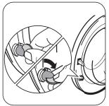
To activate this device, rotate the button (without pressing it) inside the door clockwise until the groove is horizontal. If necessary use a coin.
