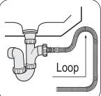
If the outlet spigot has not been used before, remove any blanking plug that may be in place. Push the drain hose onto the spigot and secure with a clip, ensure a loop is formed in the drain hose (see above) to prevent waste from the sink entering the appliance.
