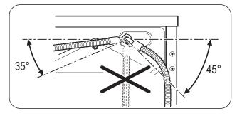
The other end of the inlet hose which connects to the appliance can be turned as showed in the picture. **Do not place the inlet hose downwards.** Angle the hose to the left or right depending on the position of your water tap. Set the hose correctly by loosening the ring nut. After positioning the inlet hose, be sure to tighten the ring nut again to prevent leaks.
