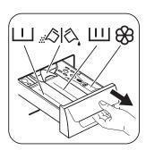
Follow the product manufacturer's recommendations on quantities to use and do not exceed the **«MAX»** mark in the detergent dispenser drawer. Any fabric softener or starching additives must be poured into the compartment before starting the wash programme.
