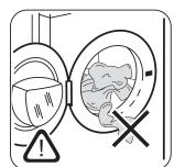
Make sure that no laundry stays between the seal and the door. There is a risk of water leakage or damage to the laundry.
