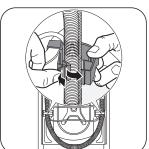
Remove the power supply cable and the hoses from the hose holders on the rear of the appliance.
