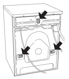
• First remove the screws and remove the washers.
