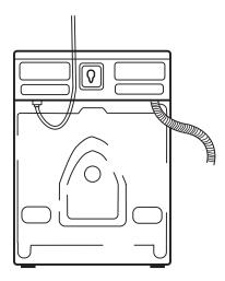
Only use the inlet hose supplied with the machine. Do not reuse old or other loose inlet hoses.
