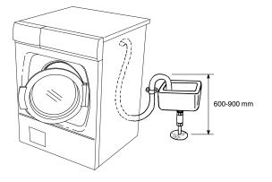
The machine can also be connected to the drain via a spigot connection. In this case the hose should also be 600-900 mm above the floor. The internal diameter of the hole should be at least 18 mm.
