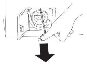
• Insert the handle back into its slot and screw it tight. Close the hatch to the drainage pump.
