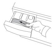
The card will then bend slightly and you can easily remove it. To fit the card, bend it slightly in order to easily insert it into the holder in the detergent compartment.
