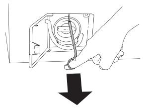
Insert the handle back into its slot and screw it tight. Close the hatch to the drainage pump.
