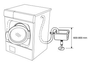
The machine can also be connected to the drain via a spigot connection. In this case the hose should also be 600-900 mm above the floor. The internal diameter of the hole should be at least 18 mm.
