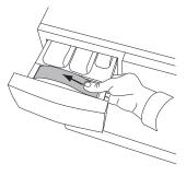
The card will then bend slightly and you can easily remove it. To fit the card, bend it slightly in order to easily insert it into the holder in the detergent compartment.
