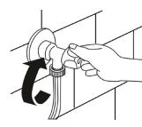
Turn off the water inlet before starting the maintenance and cleaning of your machine.
