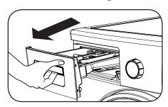
• Press the region shown below inside the detergent drawer you have pulled all the way back, and continue pulling and remove the detergent drawer from its place.
