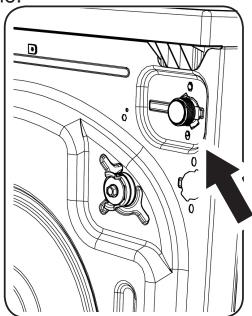
Remove the filter of the water inlet valve on your machine with a pair of pliers. Clean thoroughly using water and a brush.
