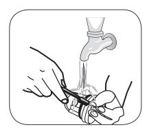
• Clean the foreign materials inside the Iter with the help of a brush.
