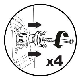
Transport screws should then be removed by pulling them out. The removed transport safety screws should be stored to be used again in case the machine needs to be transported again, e.g. if moving house.
