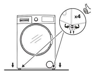
Do not install your machine on a carpet or such ground that will block ventilation from the base.
