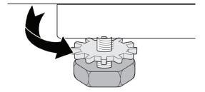
• Tighten the plastic adjustment nut after balance is achieved.
