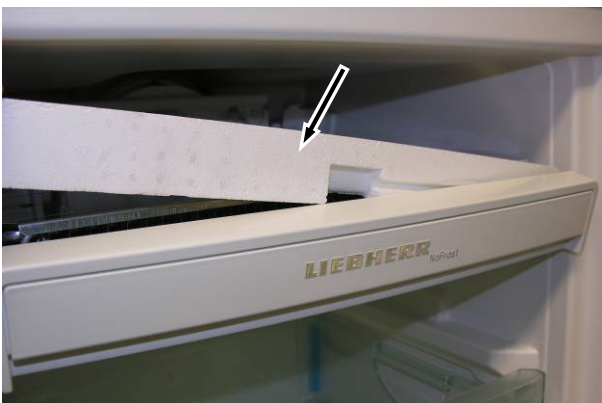
Fig. 5.2.3/ 1 Removal of the polystyrene
