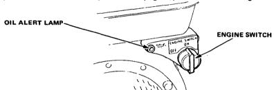
NOTE: The engine switch will remain in the ON position if the engine is stopped by the Oil Alert System.
