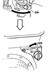
(4) Move the choke lever to the CLOSED position.
