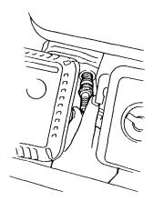
7. After a new spark plug has been seated by hand, it should be tightened 1/2 turn with a wrench to compress its washer.
