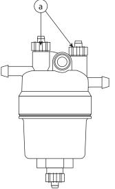
Figure 6.1 – Example of pre-filter / water seperator
