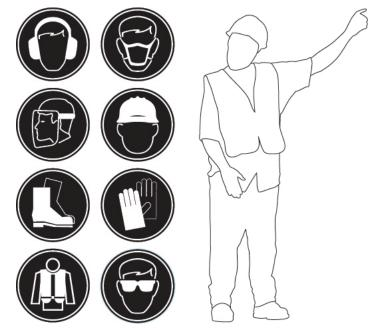
Figure 2.1 – Typical PPE to be worn by an Operator
