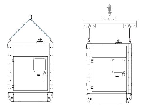
Figure 4.7 – Two Point lift
