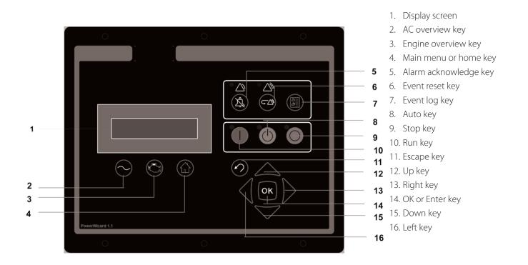
Figure 5.4 – PowerWizard Control Module Description
