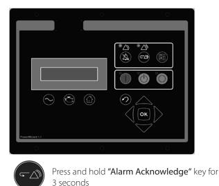
Figure 5.8 – Basic Operation Fault Alarm Reset Process
