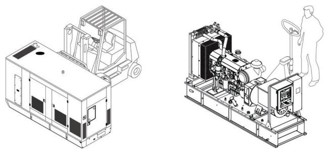
Figure 4.4 – Transporting a generator set using a forklift truck and forklift trolley
