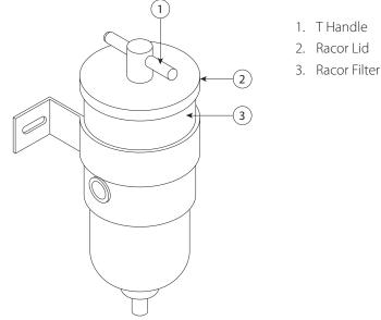
Figure 6.2 – Example of a Racor
