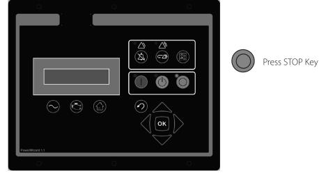
Figure 5.6 – Basic Operation Stop Key
