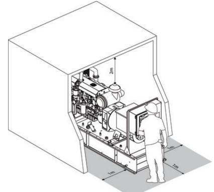
Figure 4.2 – Typical installation showing generator set access and operator workstation
