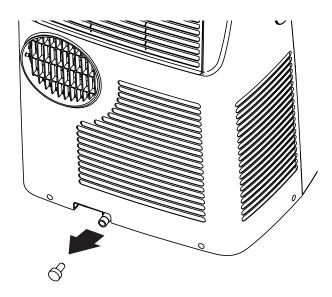
When the appliance is empty, replace the caps. Clean the filter and dry thoroughly before putting back.
