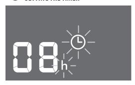
The timer can be used to delay appliance start up or shutdown. This avoids wasting electricity by not operating the appliance when it is not needed.
