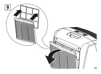
Use a vacuum cleaner to remove the dust collected on the filter. If it is very dirty, immerse in warm water and rinse a number of times. The water should never be hotter than 104°F (40°C). After washing the filter, allow it to dry completely before repositioning it.
