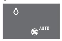
Ideal to reduce room humidity (spring and autumn, damp rooms, rainy periods, etc). In dehumidifying mode, the appliance MUST be set-up in the same way as for air conditioning, with the air exhaust hose (B2) attached to enable the moisture to be discharged outside. To set this mode:
